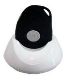
• The red light on the charging cradle remains lit when charging. The light dims or disappears when fully charged.
